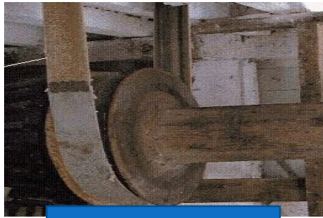
Sack Hoist Drive
